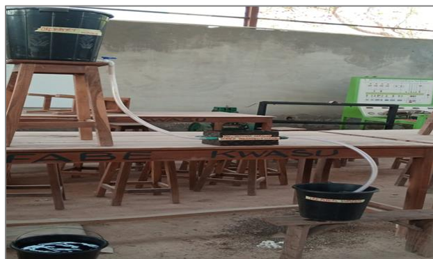
Figure 4: Neodymium magnetic treated water set up (Adopted from fieldwork)
