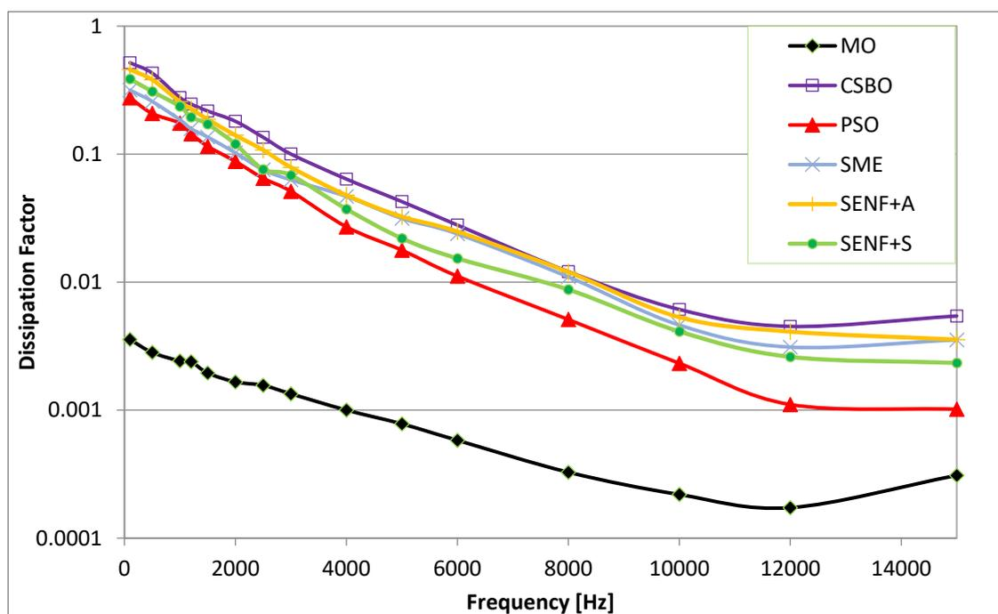
Figure 4. Dielectric loss characteristics of the oil samples at 25 °C
