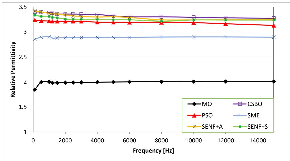
Figure 3. The frequency dependence of dielectric constant in the range of 100 Hz to 15 kHz 25 °C
