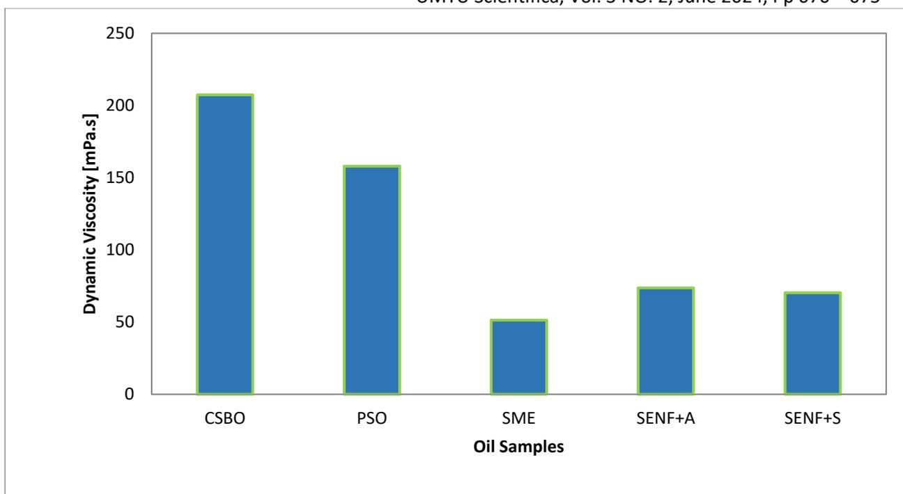
Figure 2. Measured dynamic viscosity of the oil samples at 30 °C
