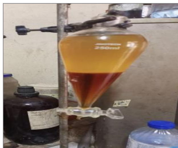
Figure 1: The Produced Biodiesel after Transesterification process undergoing separation
