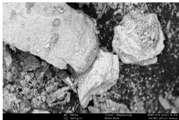
Figure 6: SEM image of ACBC after adsorption
