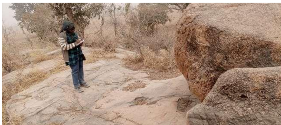
Figure 40: Photograph of non-systematic joints on Porphyritic granite (>alkali feldspar) at Garin Rau. Latitude 11° 25' 22" N and Longitude 08° 16' 52" E.
