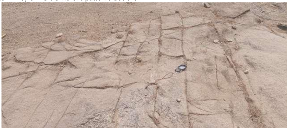
Figure 39: Photograph of systematic joints on Medium-coarse grained granite at Mahangi. Latitude 11° 14' 38" N and Longitude 08° 15' 21" E.
