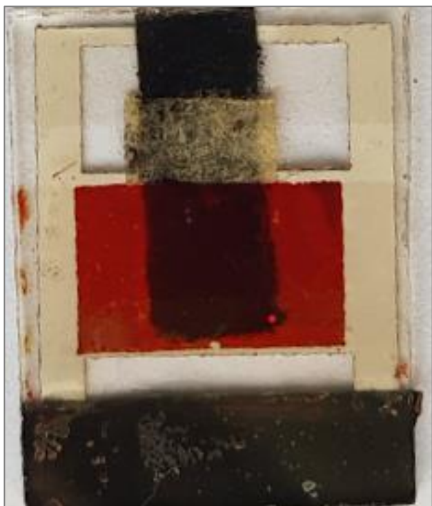
Plate 1: The fabricated \text{Cu} / \text{Cu}_2\text{O} / \text{ZnO} / \text{FTO} tandem Cell Structure
