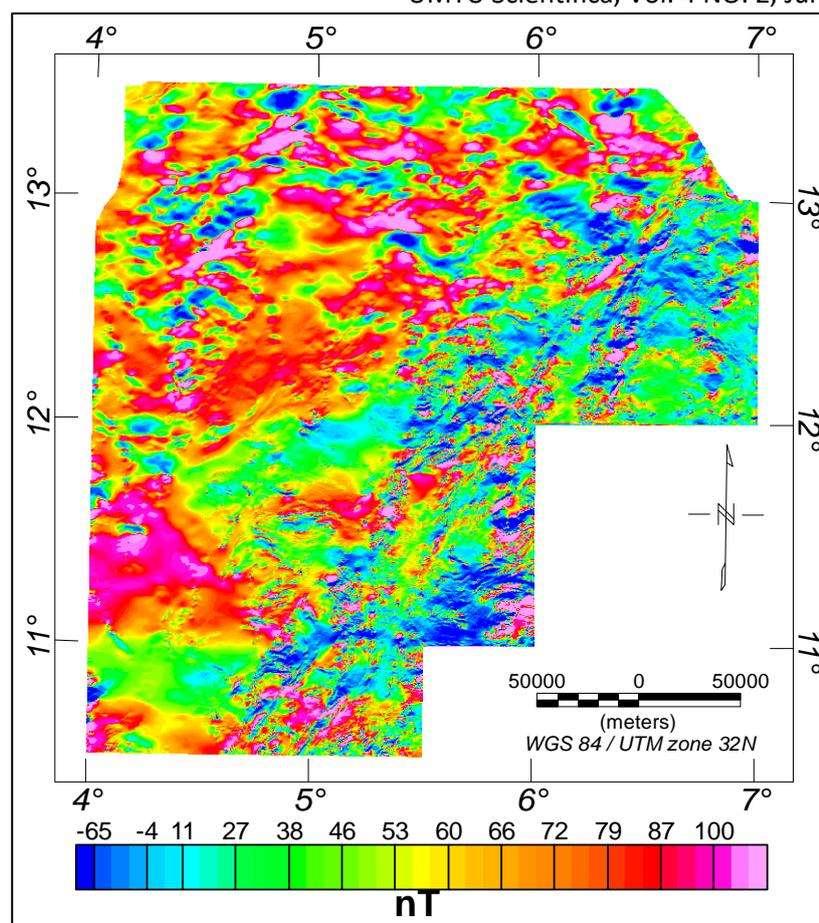
**Figure 3: Reduced to equator of total magnetic field intensity (RTE-TMI) map of the area**
