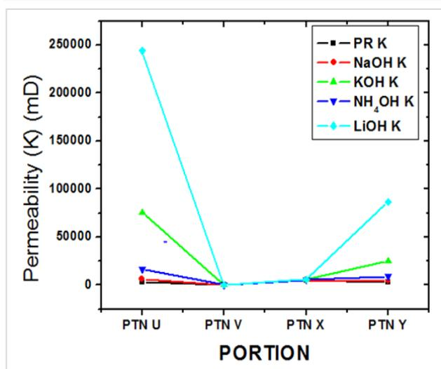
**Figure 4: Comparison of the PR K and the EOR K**
